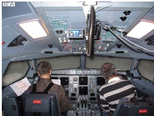
Figure 9 : The camera installed in the A330 simulator
