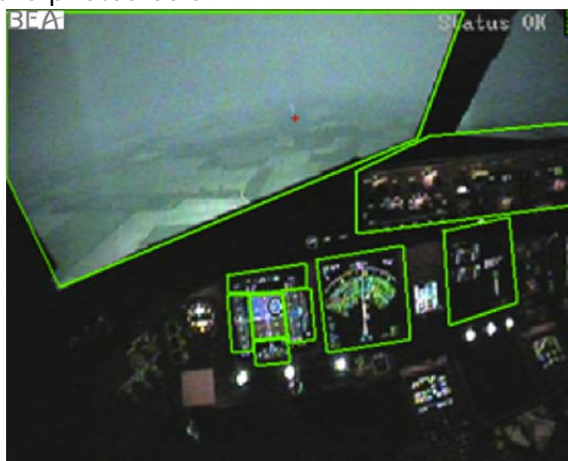
Figure 19 : definition of the zones of interest in the cockpit
